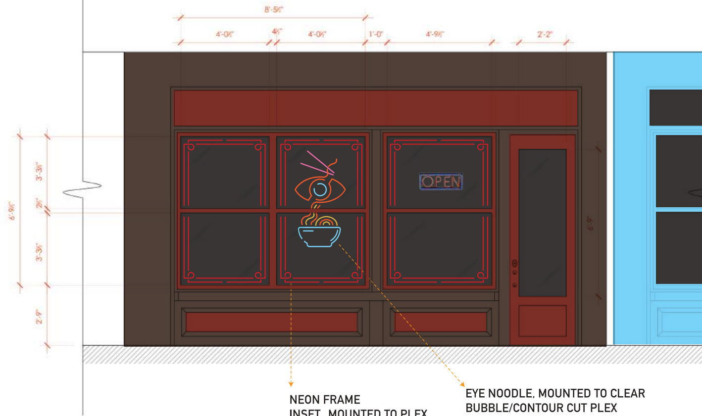
I/E. LATE NIGHT DINER - EXTERIOR FRONT ELEVATION SCALE: 1/2" = 1'-0"
